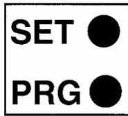
SET - On when Profile Set Mode is entered; flashes when viewing parameters in Configuration Mode after entry from Base Mode.
