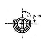
Recalibrating the temperature controller (Tools needed: screwdriver,  $\frac{3}{16}$ " open end wrench,  $\frac{3}{64}$ " Allen wrench)
