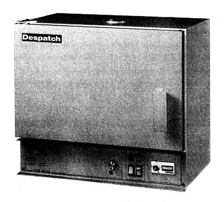
LDB series Despatch ovens are bench ovens to 204°C (400°F) with forced convection airflow.
