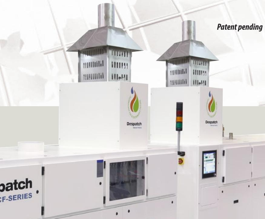
*The operation of the VOC Thermal Oxidizer is based on the principle of combustion which is the most commonly used method to control emissions of organic compounds and is used in a variety of industries. Combustion systems are simple and have very high destruction efficiency.*
