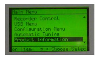
4. Press  $\square$  Four time to the screen that shows the Firmware level.
