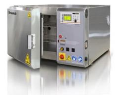
Warning: Despatch Stackable Clean Room Ovens are not to be used with flammable solvents, combustible materials or enclosed containers. If your process involves flammable solvents, consult factory about modifications.
