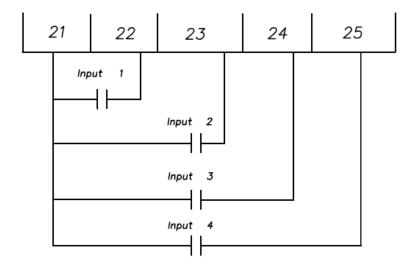
Figure 1: Digital Input Wiring
