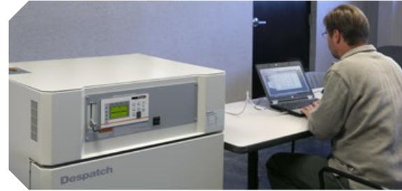
Protocol Manager™ software enables communication and control between a personal computer and up to 32 Despatch ovens equipped with Protocol 3™ or Protocol Plus controllers. The user friendly software allows oven control, recipe download and data logging.
